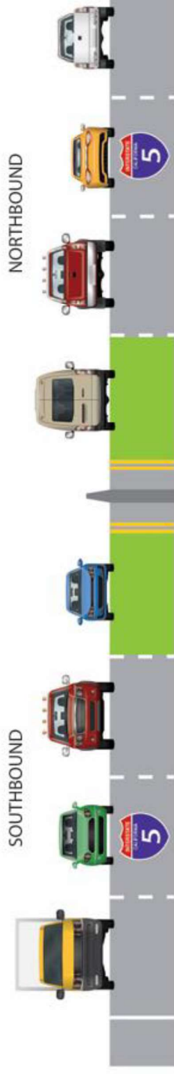
Freeway cross section between I-5/US-50 to Garden Highway. Auxiliary lanes are not shown.
